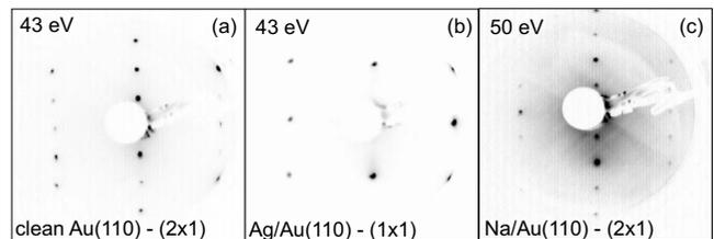
FIG. 8. LEED images of a clean  $(2 \times 1)$  reconstructed Au(110) surface,  $(1 \times 1)$  unreconstructed 1 ML Ag/Au(110), and  $(2 \times 1)$  reconstructed Na/Au(110).
